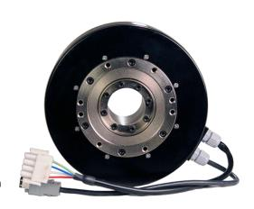
The chief advantage of direct drive products is the ability to attach a load directly to the servo motor, allowing a full range of motion control without the need for a shaft coupling or gearhead. SGM7F also offers a superior level of torsional stiffness and virtually eliminates mechanical backlash. This yields an output that minimizes damage to components and maximizes positioning accuracy and repeatability. The SGM7F also offers a host of other advantages, including:
